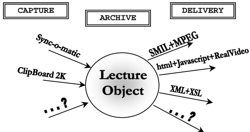
**Figure 5:** The Lecture Object architecture is based on three steps: Capturing, Archiving and Delivering. Different capturing tools, optimized to work in a certain scenario, produce standard Lecture Objects. The lecture objects are archived in a repository and are available to be used by software agents, for example a transformation to a presentation format, indexing software, etc.... The adoption of a standard format allows interoperability.
